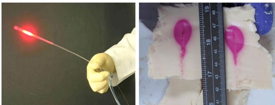
**Fig. 9** Side-firing laser fiber (left) and the ablation zone in a thermochromic phantom (right). Courtesy of Xu, et al. Xu. S.; An MRI guided system for prostate laser ablation with treatment planning and multi-planar temperature monitoring. *SPIE*. 2016;9786doi:<https://doi.org/10.1117/12.2216084>, with permission
