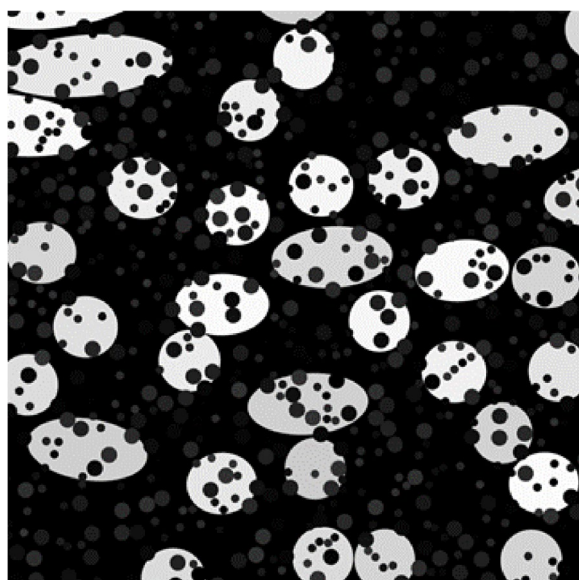
Fig. 3 An example of the synthetic training data for the network. The white ellipses mimic the fibres, the grey ellipses noise and the black background the matrix
