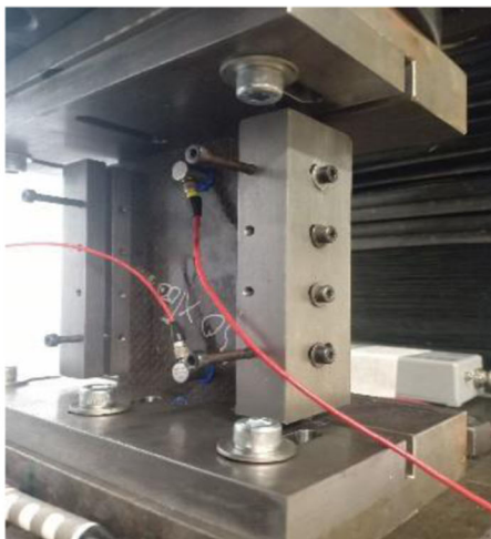
Fig. 12 a) Specimen in loading under compression b) Stress-Strain curve of REF and TUF green biocomposite
